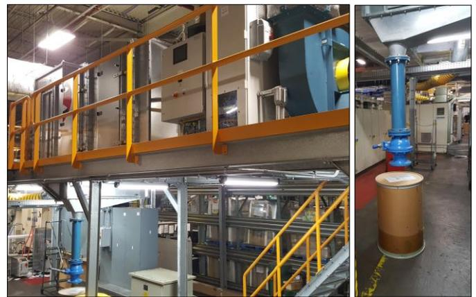
Standardized systems based on the Pusonics (Madrid) high power stepped-radiation-plate transducers (excellent directional control) are designed and engineered. This allowed successful operation of high-end extraction systems in a process exhaust air capacity range from 10.000-50.000 m<sup>3</sup>/hr.
