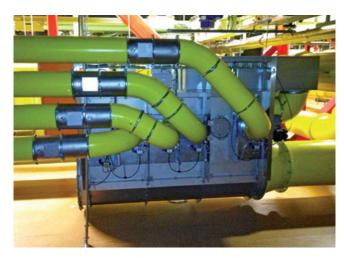
The JOA Carrousel minimizes uncontrolled maker stops, by eliminating header pressure fluctuations (see graph below).
