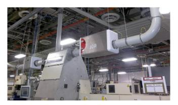
The  $\triangle VAT^{TM}$  Sensor combines an advanced optical sensor with high precision static pressure measurements, for real time data processing applying embedded hardware (FPGA – DSP).
