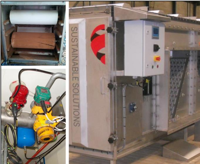
The robust, low maintenance JHF-BELT FILTER, integrated with the JOA fire extinguishing system.
