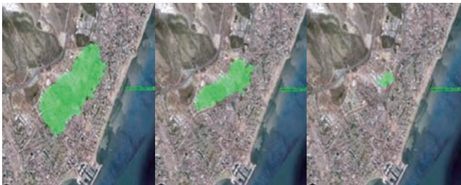
Odor contour modeling; dispersion of odors translated to the impact values at the plant contour
