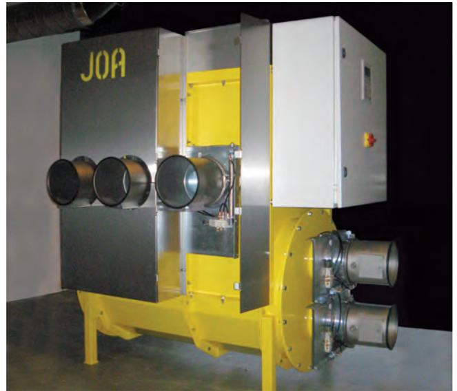
The JOA Carrousel™ minimizes uncontrolled maker stops, by eliminating header pressure fluctuations (see graph below).
