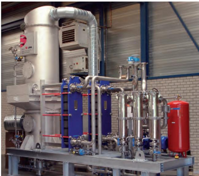
JOA ERD™ Scrubber Skid; combining exhaust-gas / steam cleaning with direct hot water or steam generation.
