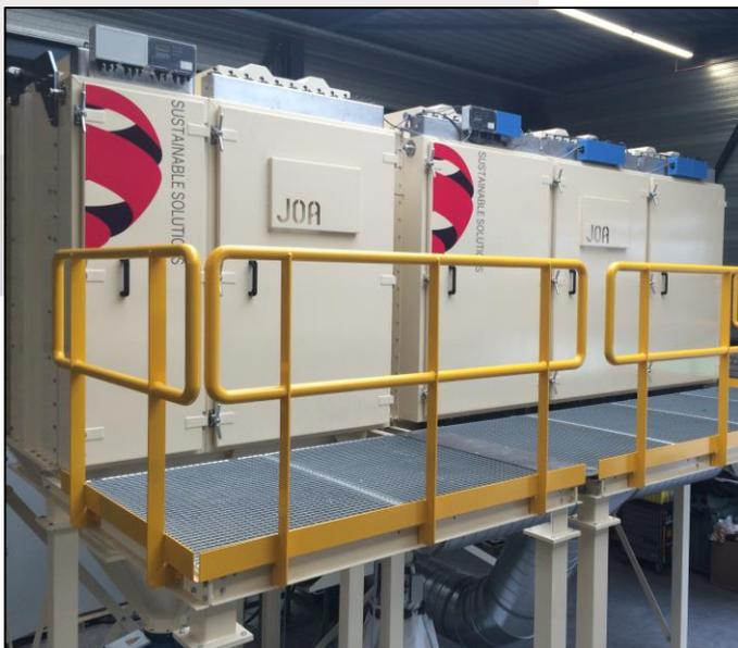
JDF Dust Filters can be equipped with integrated down-flow and / or pre-separators, providing suitable dust collection for many different applications.
